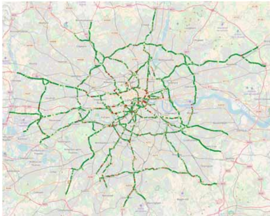
Pavement condition in Greater London, 2014
